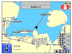
Navigating to a fishing spot using course line and Overlay Data boxes, seen in lower right corner. From top to bottom, they are: bearing, course, track, off course and steering arrow/distance.
